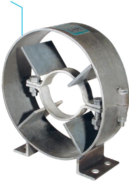
**Note:** Spider attachments to pipe must be properly located during installation to insure that a minimum of one-half the spider width remains within the length of the outer housing for all conditions of operation. See table on opposite page for maximum recommended travels. If larger travels are required, special guides can be furnished to special order.
